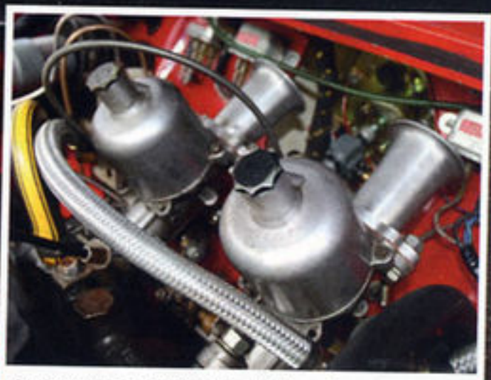
Twin SU competition H4 carbs breathe through ram pipes which are great for performance, but not so good in dusty conditions
