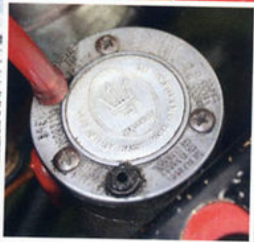
Air horn compressor ensures a healthy warning
