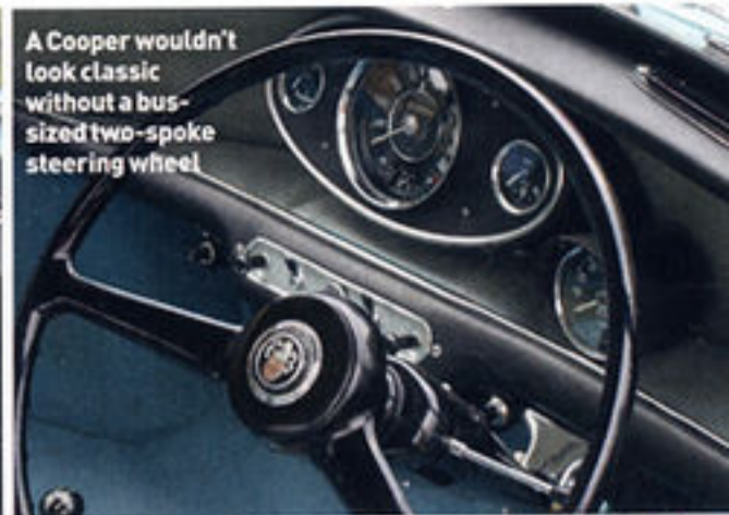
100mph Smiths speedo was only fitted to the Cooper
